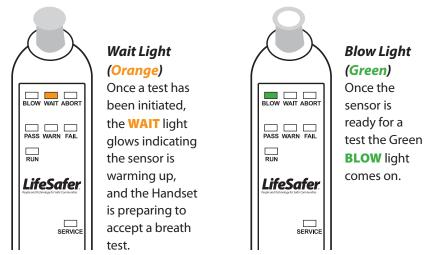
**NOTE:** Under normal operating conditions, the WAIT light stays on momentarily while the sensor warms up. If you are operating your Device in extremely cold temperature conditions (-40°F), the Device can take up to 4 minutes to warm-up.
