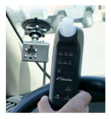
The LifeSafer FC100 with Camera System Handset is controlled by the Camera. The Camera must detect your image and "see" the target on the back of the Handset before it will allow you to take a test. Hold the Handset 4-8 inches from the front of the Camera module in order to get the Camera to release the Handset for the test.
